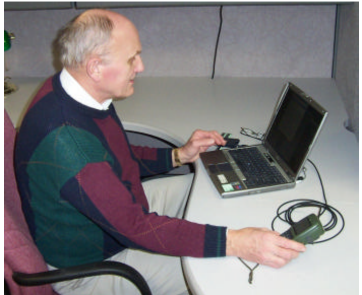
Bill Pohlmann, ARINC Engineer at PM GPS Fort Monmouth reprograms a DAGR using software files downloaded from the GPS website to a laptop and a DAGR-PC interface cable. The process takes a couple of minutes per DAGR.
